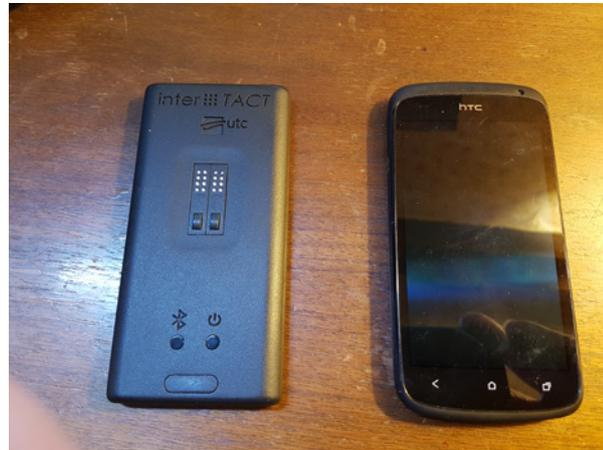
The Touch Interaction Module integrates 16 piezoelectric pins. It connects to a smartphone via Bluetooth and can be attached to the back of the smartphone.
