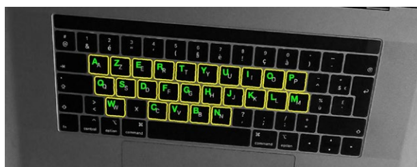
Image of a French language (azerty) computer keyboard (GoPro 9, resolution 1080 x 1920 x 3, 200 frames per second). The identity of the letters on the keys is correctly defined (letters in green), except for the X key. Keys with symbols other than capital letters are correctly excluded. The outline of the keys is correctly marked (yellow lines).
