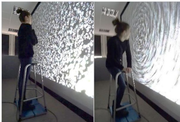
Figure 1: The PIVVIT platform, a large VR-based field-of-view device using optic flow to stimulate the vision-balance interaction in therapeutic protocols.
